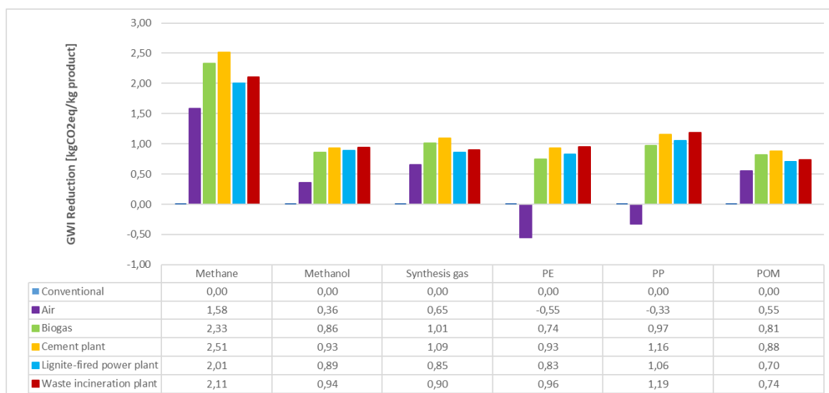
Figure 16: GWI reduction potential for the production of basic chemicals and polymers from different CO 2 sources compared to the conventional method (based on Hoppe et al., 2017)
